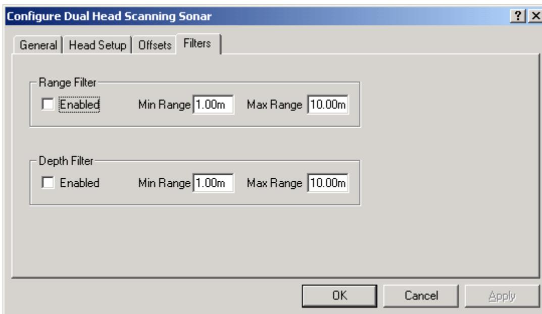
In the Filters tab you can enable the Range and Depth filters by selecting the appropriate checkbox. These filters function as gates where you enter the minimum and maximum expected Range/Depth values and WinFrog will discard any data that falls outside of the specified ranges.
