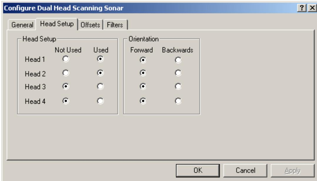
In the Head Setup tab, the Head Setup section allows you to select those heads that are to be used. If the data for a scanning head is to be used, and logged to a raw file if raw data logging is active, it must be selected as *Used*. Selecting *Not Used* results in the data from the driver for that head not being passed to the vehicle that the data item is associated with and is therefore neither used nor logged to the raw file.
