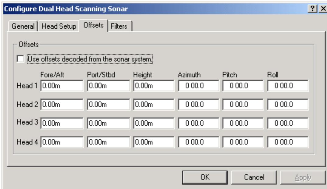
In the Offsets tab you have two options for applying offsets. By selecting the Use offsets decoded from the sonar system checkbox, WinFrog will use the offsets as entered in the control unit. These offsets are included in the data string from the control unit. Alternatively, you can leave that checkbox unselected and enter the offsets manually.
