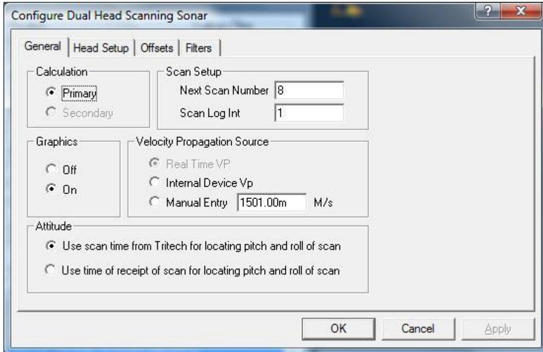
In the General tab, selecting either the Primary or Secondary option has no effect on the operation of this device or the data collected.
